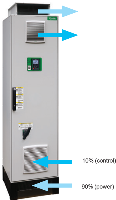
Cooling system with two separate air flows
