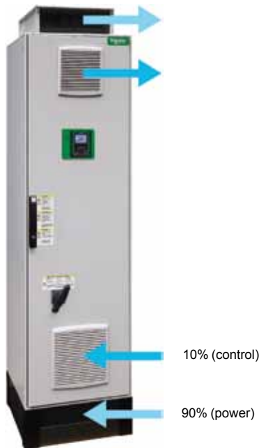
Cooling system with two separate air flows
